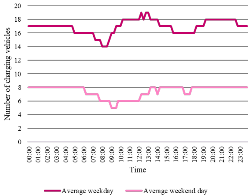
Figure 11 Occupancy in number of fast roadside charging sessions over an average day.
